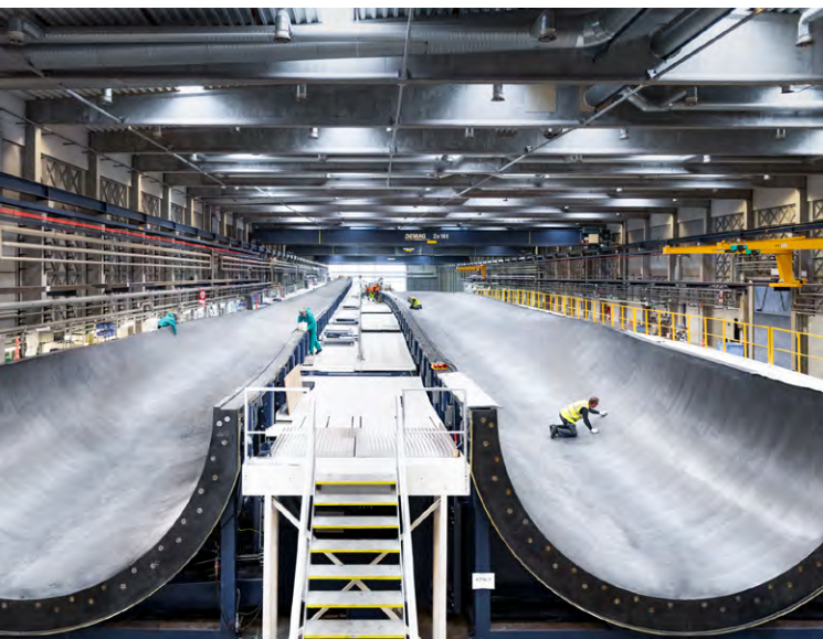
↑ The offshore turbine, V236-15,0 MW™, is moving closer to realisation. Once the prototype is ready, it will be installed at the Østerild National Test Centre. The blade mould has already been installed at the blades factory in Nakskov, Denmark.
